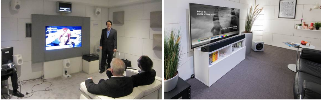
Figure 5. First (left) and second-generation (right) 3D soundbar designs. Wall mounted speakers in the left photo were used for discrete playback to simulate professional monitoring and enthusiast listening.
