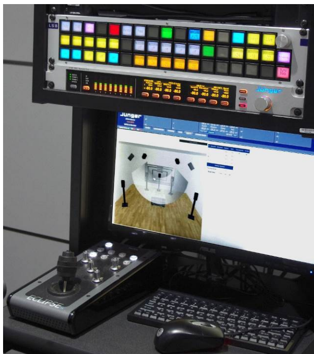
Figure 3. Junger Audio MPEG-H Audio Monitoring and Authoring Unit
