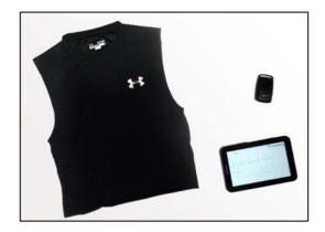
The FitnessSHIRT reads out physiological signals like pulse and breath continuously when worn. The interpreted data can be viewed on a smartphone or tablet PC, for example. © Fraunhofer IIS | Picture in color and printing quality: www.iis.fraunhofer.de/press.
