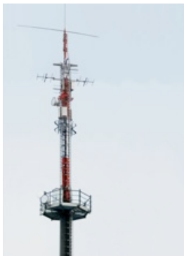
One of the two base stations for the test bed located at Fraunhofer IIS in Erlangen. © Fraunhofer IIS/Hans Adel | Image in color and print quality: www.iis.fraunhofer.de/pr .
