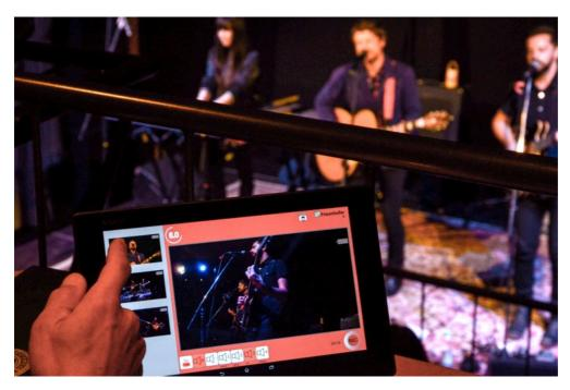
The HIGGS multi-camera video system from Fraunhofer IIS enables live streaming by using up to five portable cameras and a flexible, easy-to-use video-editing app.
