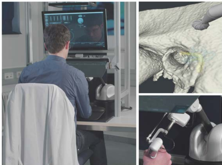
“HandsOn.surgery” trainer: virtual bones with risk structures and surgical bur (top right), haptic arm for virtual milling (bottom right).
