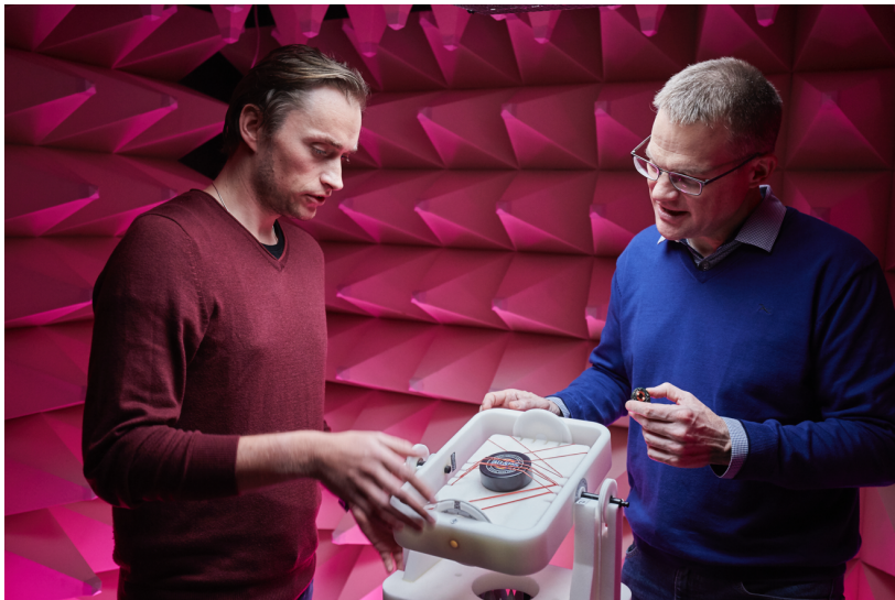
The tracking system measures the position of the puck 2000 times per second. © Fraunhofer/Piotr Banczerowski
