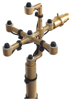
Figure 9. Microphone Array for Automatic Speaker Measurement (including Angle and Distance)
